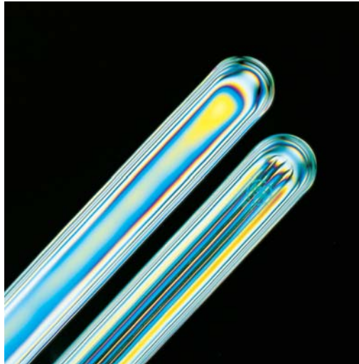
KLINGER transparent glass (left side) and reflex glass (right) in polarized light
